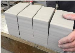
Extrusion and cut to the final shape
