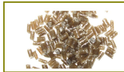
Compound PA6/Basalto in granuli
